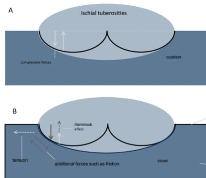
Figure 1 Theoretical model of hammock effect in wheelchair cushion. (A) The situation without a cushion cover, (B) The situation with a cushion cover. Friction from the cover develops causing additional tension along the cushion surface producing forces known as the hammock effect (Iizaka et al, 2009)
